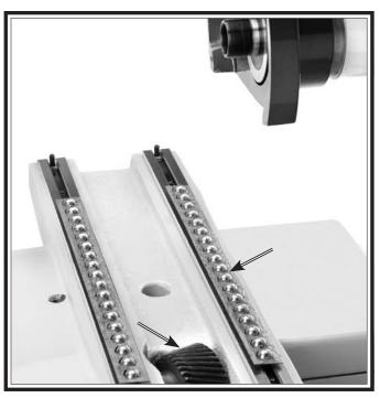
Figure 40. Ball bearing ways.
